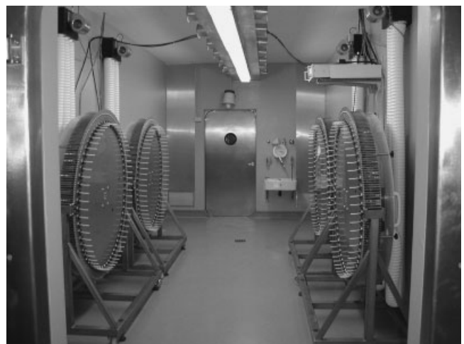
Fig. 1. Exposure setups. One of two animal rooms with an exposure system for mice (i.e., GSM [902 MHz] or DCS [1747 MHz]) consisting of four wheels, three for the different whole body SAR levels and a sham exposure wheel, and related ventilation system.
