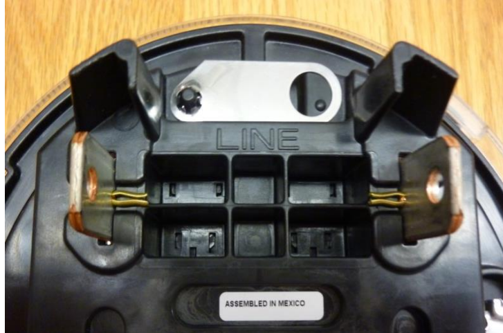
Figure 3: Holes in back facilitate mounting of various Sensus meter modules.
